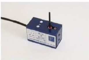
Model : WBFJ High Accuracy and "G" free Range : 0.3N~1N Accuracy : 0.035%
