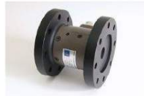
Model : TP (Reaction type) High-Capacity Range : 50Nm~20kNm Accuracy : 0.2%
