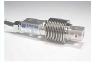
Model : WBU Beam type and Metal bellows Range : 10N~2kN Accuracy : 0.015%
