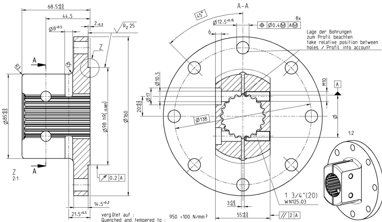
Profile sleeve 21 teeth (1 3/8''), ≤ 5000 Nm continuous dynamic load
