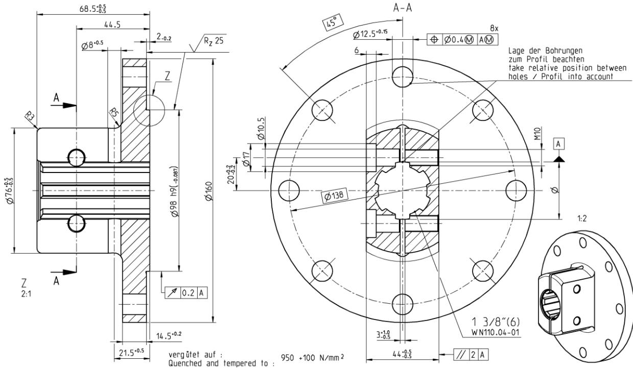
Profile sleeve 20 teeth (1 3/4"), ≤ 5000 Nm continuous dynamic load
