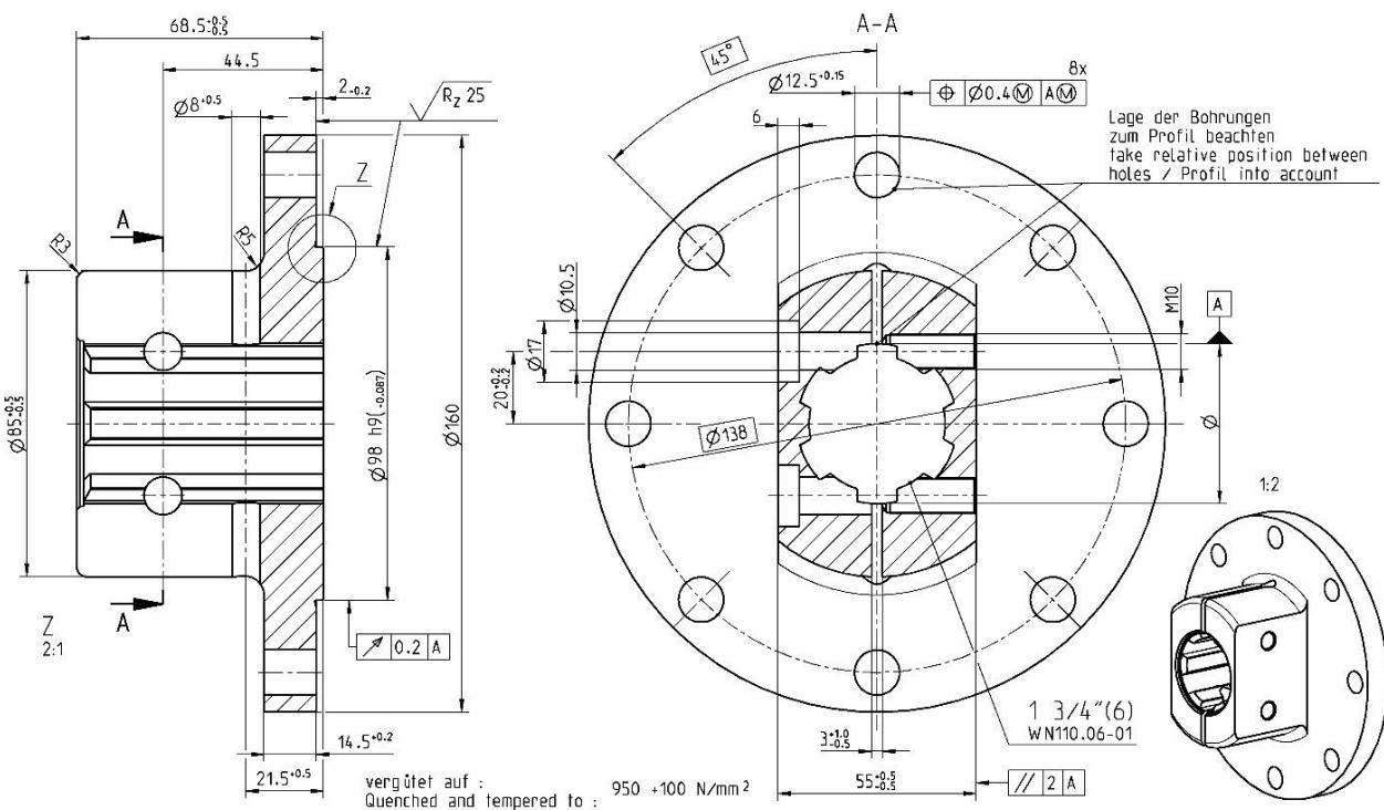
Profile sleeve 6 teeth (1 3/8"), ≤ 5000 Nm continuous dynamic load
