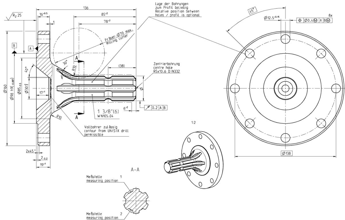
Profile shaft 20 teeth (1 3/4"), ≤ 5000 Nm continuous dynamic load
