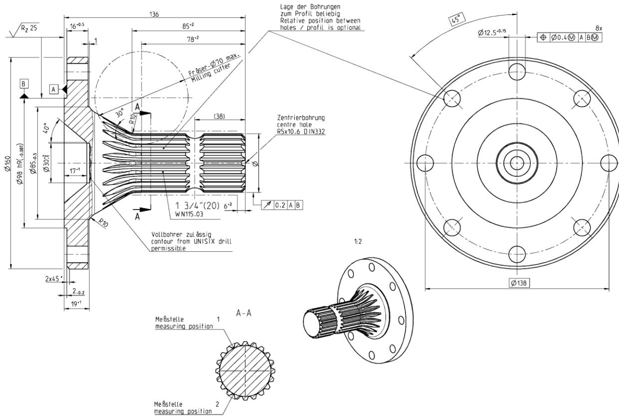
Profile shaft 21 teeth ( $1\frac{3}{8}''$ ),  $\leq 3000 \text{ Nm}$  continuous dynamic load
