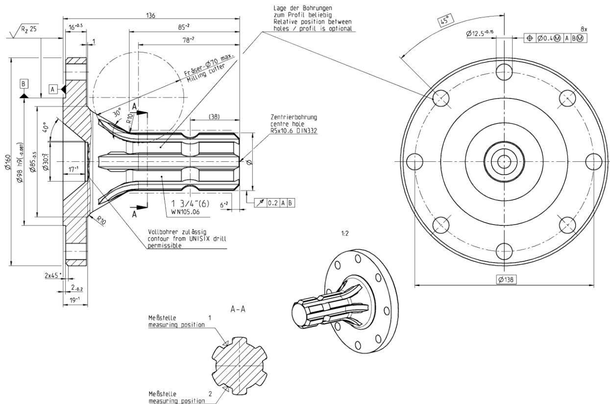
Profile shaft 6 teeth (1 3/8"), ≤ 2500 Nm continuous dynamic load
